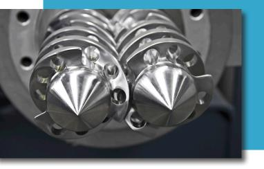
The screw geometry has been developed for a large processing window and in combination with the direct drive concept it provides a higher quality homogeneous melt. The innovative and technological features of the T-Rex extruders result in increased energy savings.
