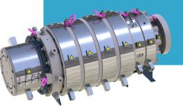
RSD die heads have been designed, using a computer calculation program based on a 3D visco-elastic model for plastics. The program calculates the optimum flow lines for compression cones that otherwise would not be feasible for reliable use in production.
