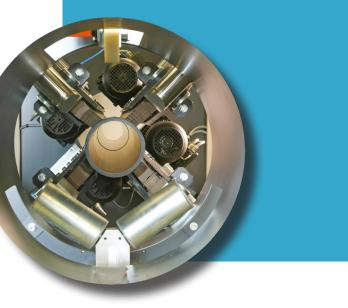
A Rollepaal haul off continuously pulls thermoplastic pipe through the cooling line after it comes out of the extruder. The tracks of the haul off are controlled by separate servo motors. Accurate and constant hauling speed is obtained
