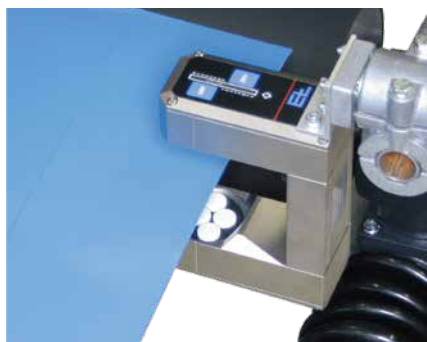
Ultrasonic edge sensor FX 5 in film manufacturing machine
