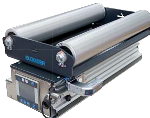
ELGUIDER DRB23 with ultrasonic edge sensor FX 46
