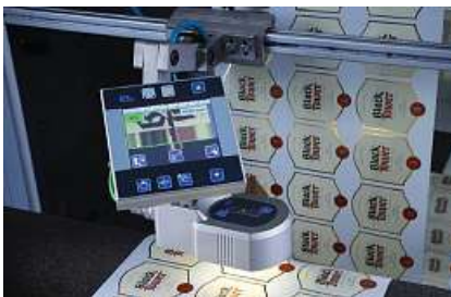
Color line sensor FE 52 on roller inspection machine
