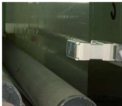
Ultrasonic edge sensor FX 5 in film manufacturing machine
