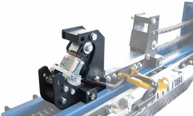
Fabric tension sensor EM 10 in the tension carriage
